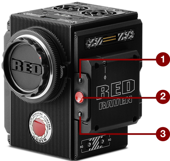
Figure: RED RAVEN Media Bay Controls
