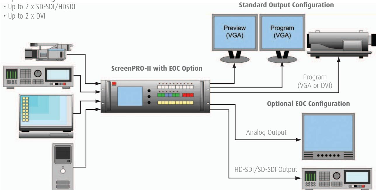
The EOC, which employs a separate Athena scaler for the optimum in image quality, derives its inputs from either the main ScreenPRO-II Program or Preview output. On the EOC connector panel, one BNC is provided for the HD/SDI output, and five BNCs are provided for analog output. Both outputs are active simultaneously — depending on the selected output resolution (see the **Specifications** page for a complete list).
