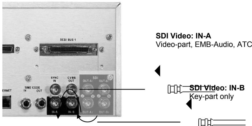
Figure 24: SDI Video Input A and B Connection
