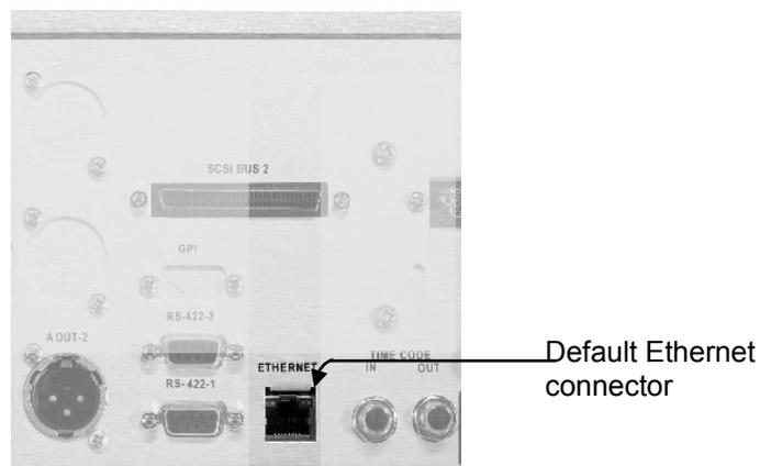
Figure 7: Ethernet Connector – Rear Panel
