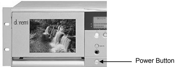
Figure 6: Power Button - Front Panel
