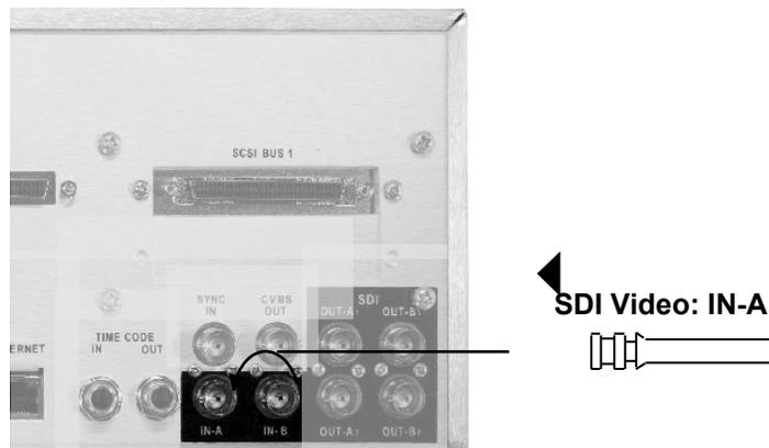
Figure 2: Video Input – V1 Rear Panel
