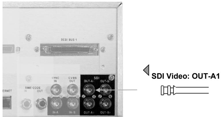
Figure 4: Video Output – V1 Rear Panel
