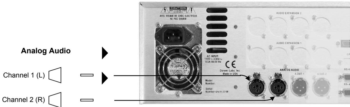
Figure 1: Audio Inputs – V1 Rear Panel
