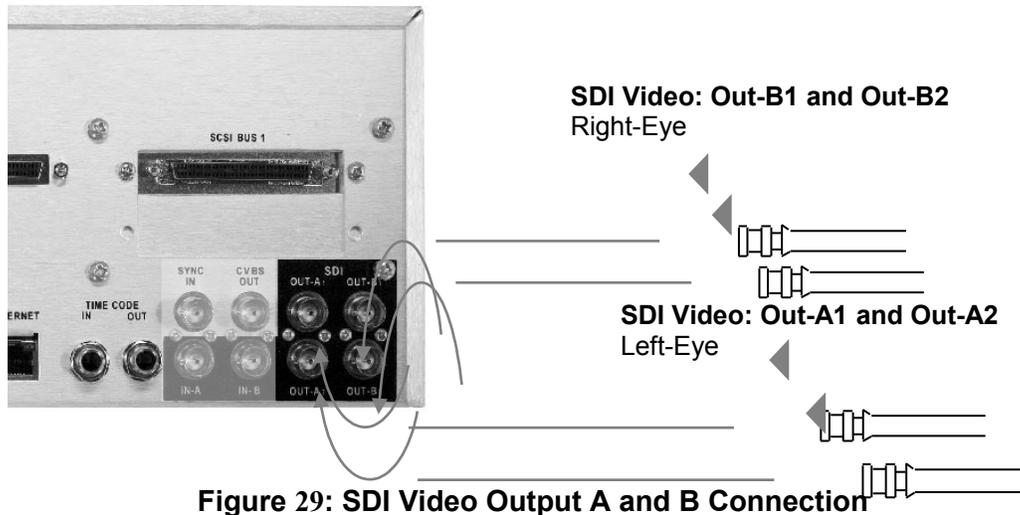
Figure 29: SDI Video Output A and B Connection
