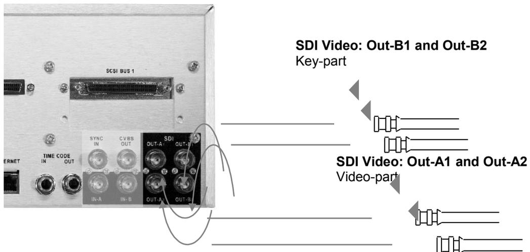
Figure 27: SDI Video Output A and B Connection
