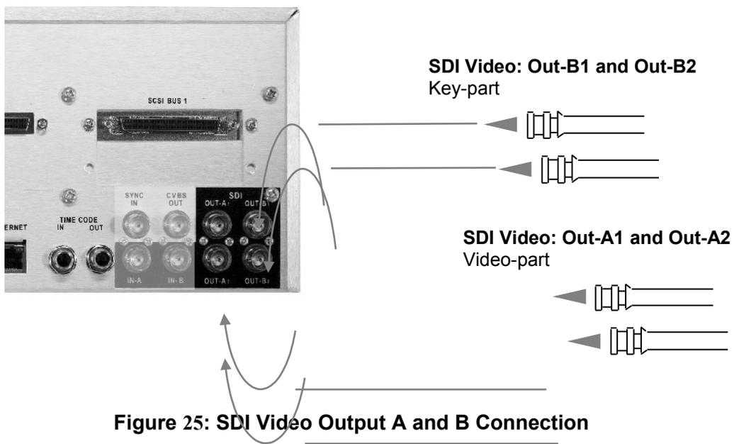
Figure 25: SDI Video Output A and B Connection
