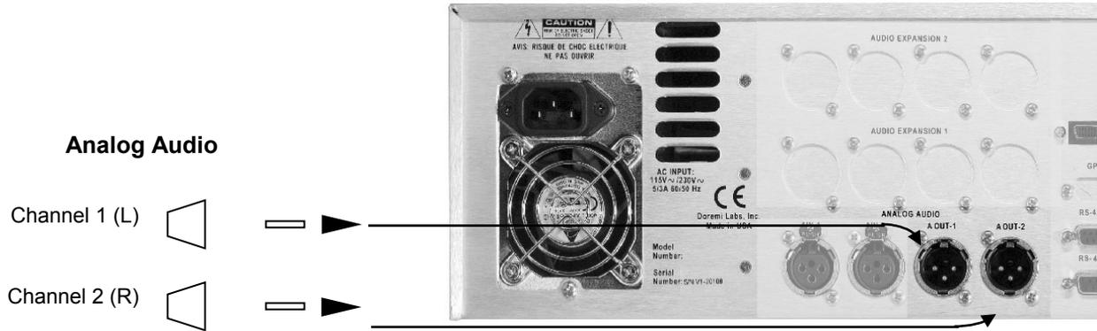
Figure 3: Audio Outputs – V1 Rear Panel
