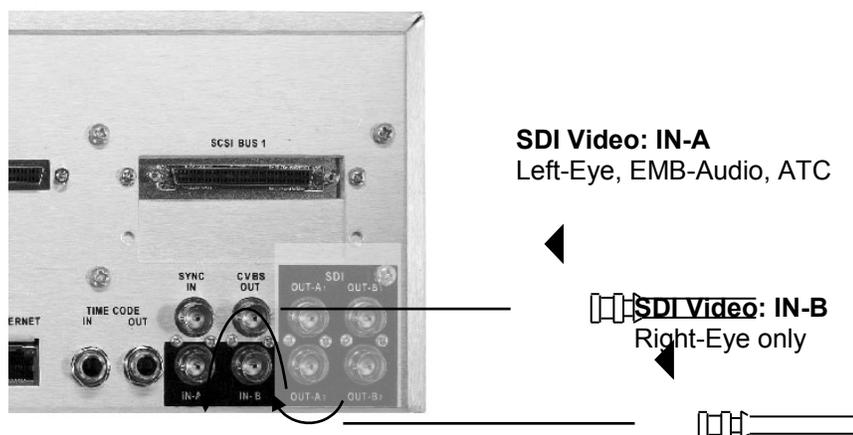
Figure 28: SDI Video Input A and B Connection
