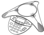
The three LEDs are red when a call is muted, and green when it is not.
