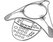
The three LEDs blink green when the phone rings.
