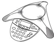
The three LEDs blink red when a call is on hold and are green when it is resumed.
