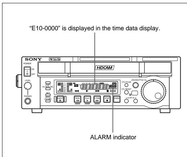
If this happens, the drum and capstan motors stop and the cassette is automatically ejected. Then, the drum starts to rotate again to dry its surface. In this state, the unit is not operable. When the moisture has evaporated, the ALARM indicator goes off and the “E10-0000” message disappears.
