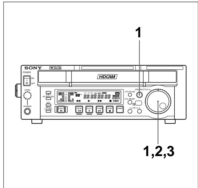
In jog mode, the JOG dial controls the playback speed based on the speed at which the dial is turned. The playback speed range is  $\pm 1$  times normal speed. Use the following procedure to carry out playback in shuttle mode.
