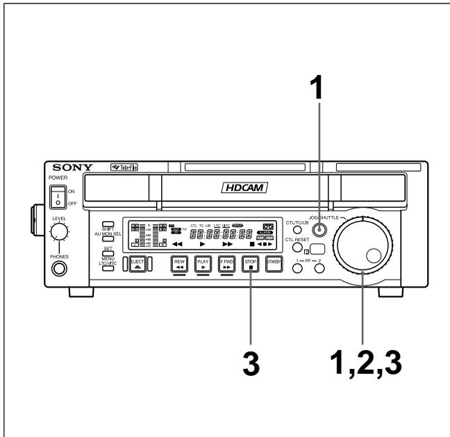
In shuttle mode, the SHUTTLE dial controls the playback speed based on the angular position of the dial. There are seven playback speeds:  $\pm 0.03$  times,  $\pm 0.12$  times,  $\pm 0.5$  times,  $\pm 1$  times,  $\pm 2$  times,  $\pm 5$  times,  $\pm 21$  times.
