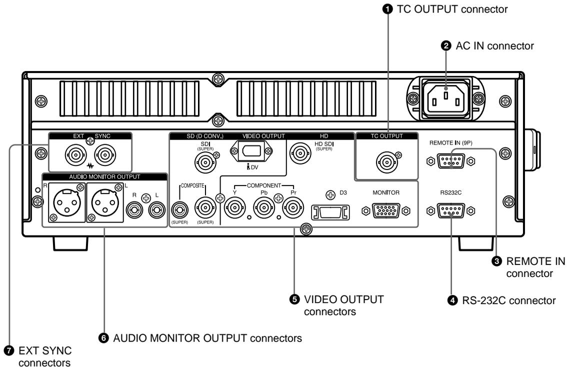
This illustration shows the J-H3 equipped with an HKJ-101 i.LINK Interface Board.
