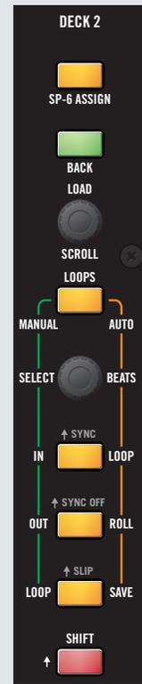
**SCROLL / LOAD** encoder: Rotate the knob to scroll through the Crate / Library panel currently in focus. When the focus is in the Crate area, pressing the knob displays the contents of the selected Crate and moves the focus into the Library area. When the focus is in the Library area, pressing the knob loads the selected track to the Virtual Deck. Double-pressing will load an instant double to this Deck from the opposite Deck.
