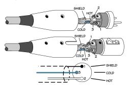
Pin 1 = Ground or shield Pin 2 = Positive (+ or hot)Pin 3 = Negative (- or cold)
