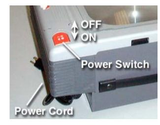
Unravel the power cord from its storage position under the front. Check that the red power switch is in the OFF (up) position before you plug the cord into a standard AC electrical socket.
