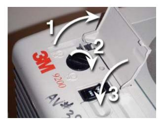
IF THE BULB SHOULD BURN OUT, lift the small gray door left of the power switch and above the 3M logo. Rotate the knob underneath to select the auxiliary bulb. Shut the gray door -- the lamp will NOT turn on with the door still open.
