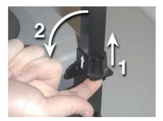
When finished, turn the projector OFF. Then, unplug it from the AC outlet and store the cord in its storage bracket under the front. Pull UP on the mirror arm's locking mechanism (indicated by a white arrow) and gently lower it into its storage/carrying position.
