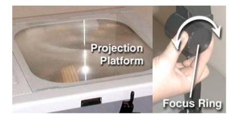
Place a transparency slide on the projection platform and aim the projected image at your screen. Please do not write directly onto the projection platform. The mirror can be tilted slightly to adjust the image height. Use the knob located on the right of the mirror arm to focus the image.
